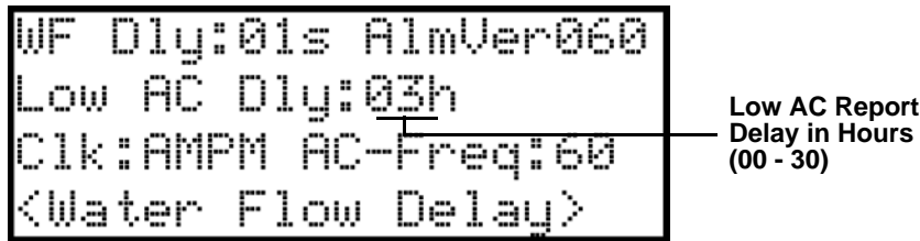
Figure 7-18 Low AC Report Delay Programming Screen
